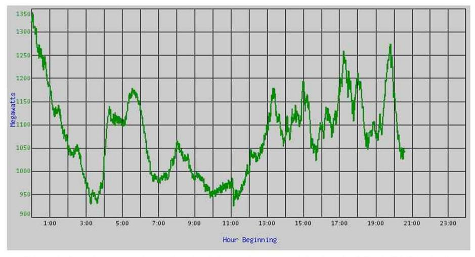
This graph shows the aggregated output from the wind generation connected directly to the California ISO Balancing Area.
