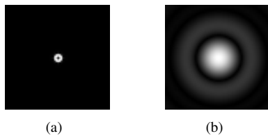
Fig. 1. Lens in (a) and the generated illumination in (b) used for ptychographic PR.
