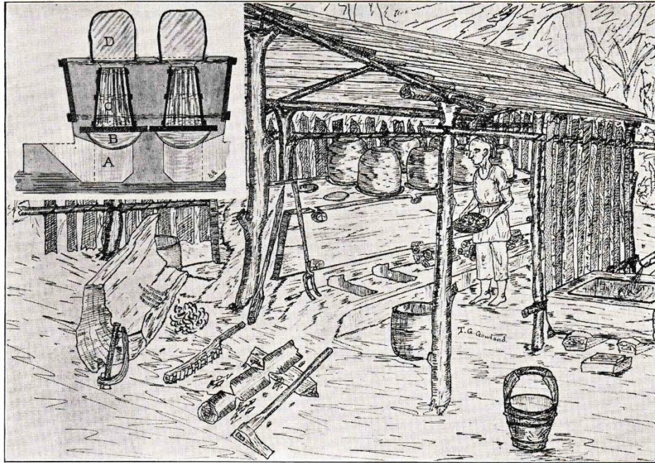
Old Model Chinese Camphor Still ("Stove") "A" Fire-box. "B" Water-pan. "C" Chip-retort. "D" Crystallization Jar.
