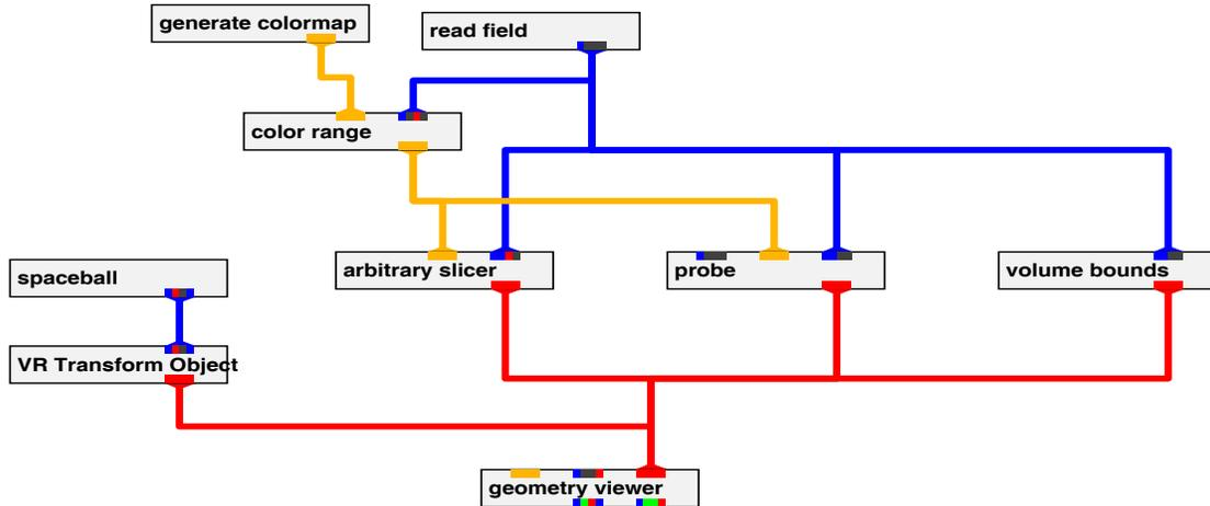
Figure 3 - VR Input Device Controls Location of Data Probe
