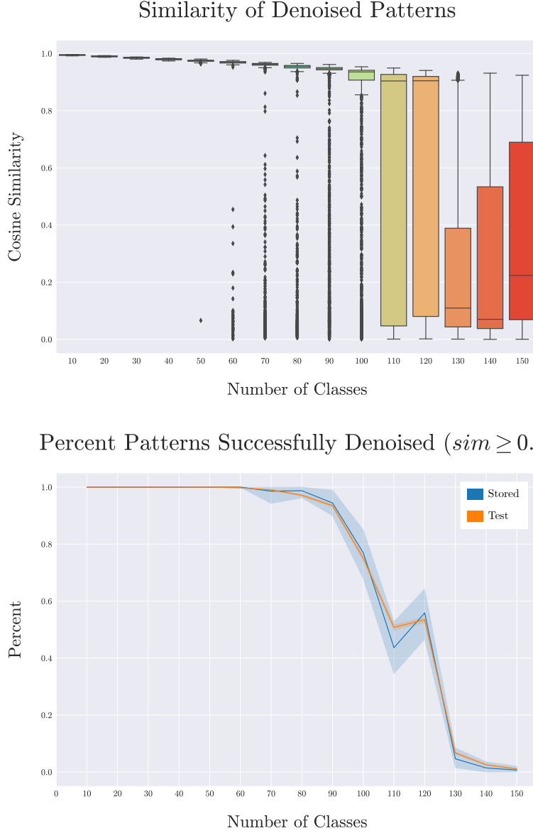
Figure 5.2: Random Phasor Orbit Denoising Performance. (Top) Cosine similarity of denoised patterns for the orbit of transformations of the stored patterns. (Bottom) Percent success (cosine similarity \geq 0.9 ) at denoising stored patterns (blue) and their transformation orbits. Bispectral Hopfield Networks successfully generalize to all transformed versions of the stored patterns, with denoising performance on the test orbit mirroring performance on the stored patterns.
