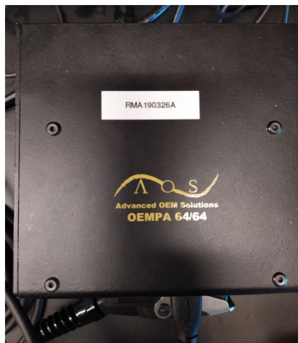
Figure 6.3.A full-matrix capture (FMC) controller.
