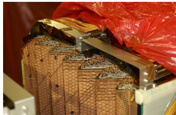
Figure 3.20: The LAr calorimeter uses an accordion geometry to provide uniform coverage in \phi . Steel-clad lead plates are interleaved with electrodes, consisting of three copper layers separated by polyimide sheets. (a) shows a schematic drawing of a LAr barrel module, illustrating the accordion geometry and the three layers in depth, with fine segmentation in \eta in the layer closest the interaction point. (b) shows a photograph of the accordion geometry.
