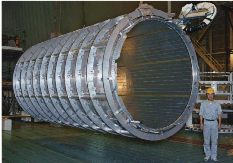
Figure 3.8: The central solenoid in the factory after completion of the coil winding [9].
