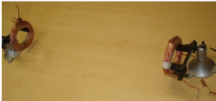
Fig 3.3 Experimental setup for near-field power transfer measurements
