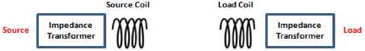
Fig. 6.4 Impedance matching scheme for 2-coil configuration: Impedance transformers with variable turn ratios
