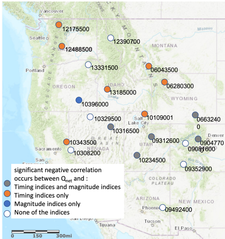
Figure 5. Distribution of four types of sites, classified by the correlation results between Q_{net} and snowmelt runoff indices. Grey points show sites with negative correlation between Q_{net} and both timing ( D_S and D_P ) and magnitude indices ( Q_S and Q_P ). Orange points show sites with negative correlation between Q_{net} and timing indices only. Blue points show sites with negative correlation between Q_{net} and magnitude indices only. White points show sites with no significant negative correlation between Q_{net} and any of the timing and magnitude indices
