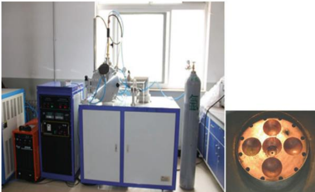
Figure 5.1.1. Arc-melting method to make high-entropy alloys [136].
