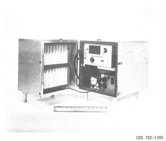
Figure 2: Photograph showing the radiometer package assembled. The unit shown in Figure 1 is located in the lower right segment of the housing in this photograph. Above it is the electronics package for the Barnes radiometer. The left hand segment contains an air blower, which is located behind the air filter shown.
