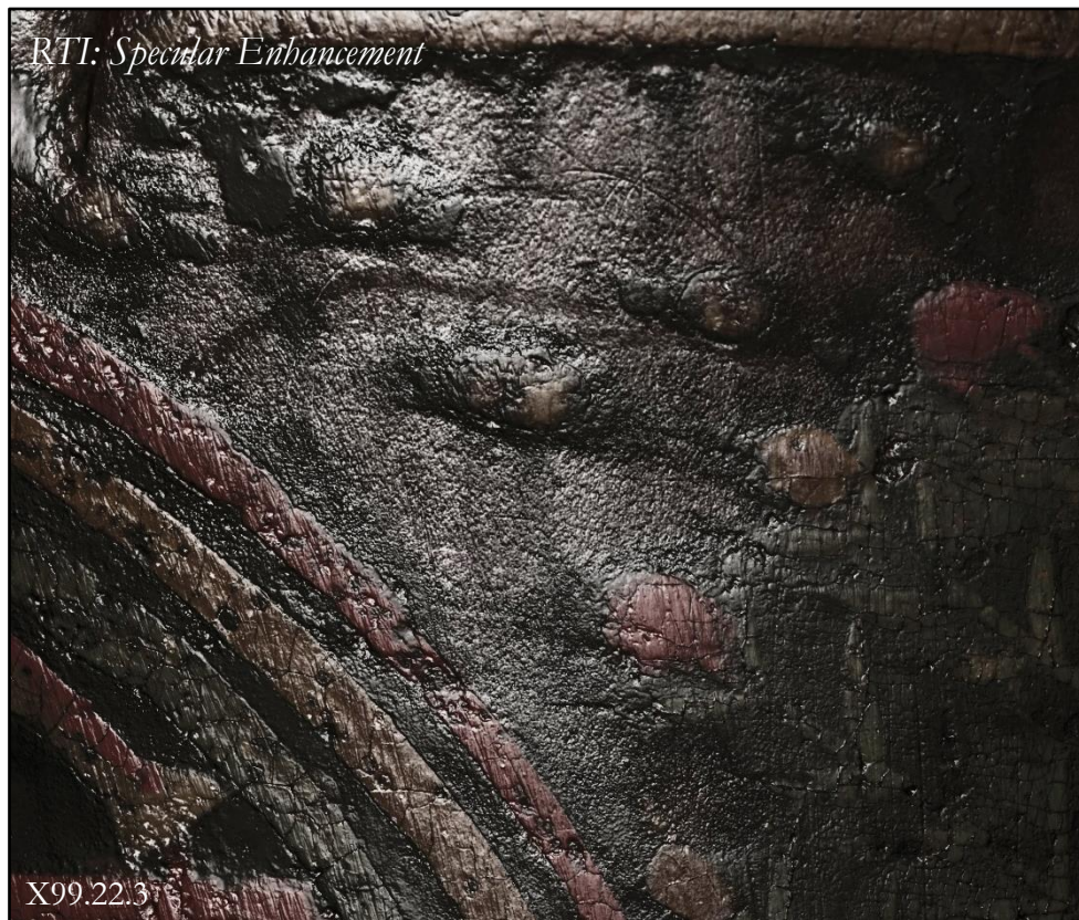
Fig. 47. RTI captured the depth of scrapes on the surface, which abruptly stop near inlay. Rendering Mode: Specular Enhancement (Diffuse Color = 40, Specularity = 70, Highlight Size = 74).
