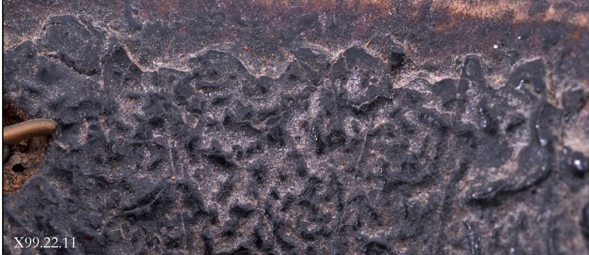
Fig. 36. Dark material on upper qero interiors often displayed a “wrinkled” surface, called blistering, following a raised network of cracks. Qero X99.22.5 appeared coated by Gloss.
