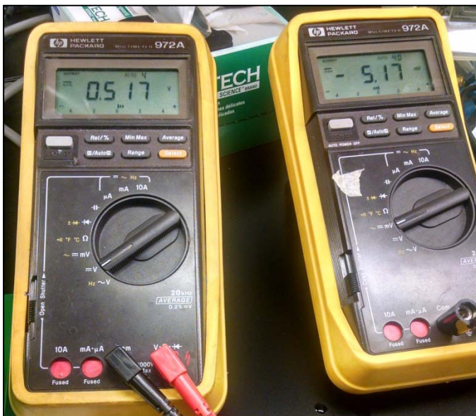
Gain set to 100 for amplifier mounted on TP1. ~1 psi load applied to pressure transducer 26PC6CF6G via vertical tube of water. (10/2014)
