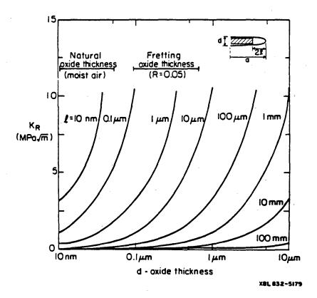
FIG. 2. Computation of the value of the resultant stress intensity  $K_R$ due to a rigid wedge of constant thickness (d) located distance 21 behind the crack tip (Eq. (1)). Calculations for steel where the elastic modulus E = 2.1 x 10<sup>5</sup> MPa and Poisson's ratio v = 0.3.
