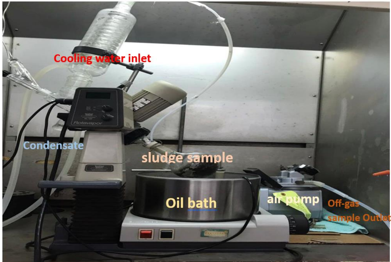
Figure 2.7. The Laboratory Rotary-Evaporator Sludge Drying System used at UCLA
