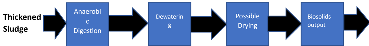
Figure 2.1. Schematic diagram of the Sludge Treatment Process
