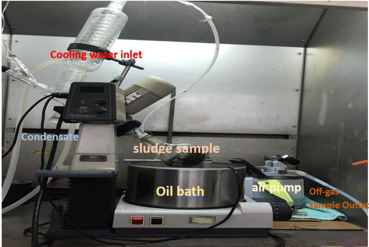
Figure 3.3. The Laboratory Rotary-Evaporator Sludge Drying System (Decottignies et al., 2010)
