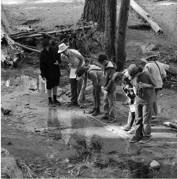
Figure 9.4 Measuring flow speed by floating leaves down a stream and timing their progress
