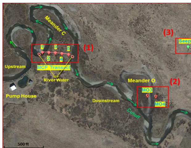
Figure 1. Sampling location for \text{H}_2\text{O}_2 detection in the East River floodplain, including three groups of sampling wells: (1) The MCP transect within the intra-meander hyporheic zone, including five piezometric observation wells (MCP1 to MCP5); (2) Two sampling wells (MO3 and MO4) close to the new river channel of Meander O (the “neck cutoff”); (3) One sampling well (Seep) at the Mancos Shale seep (approximately 150 m uphill from the oxbow lake of Meander O). Green arrows indicate the flow direction in the river. This image was acquired and modified from Google Earth , earth.google.com/web/ .
