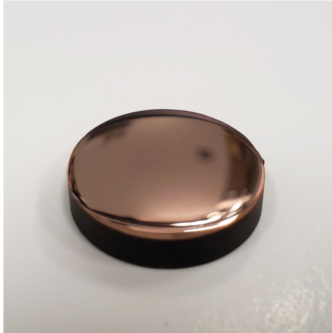
Figure 2.1: Uniform mirror finish reached on the disc top surface after being processed following the polishing routine
