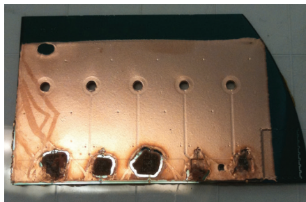
Figure 3.4: Chip after wet etch. The area around the pads, which were masked by super glue, is etched at an accelerated rate.
