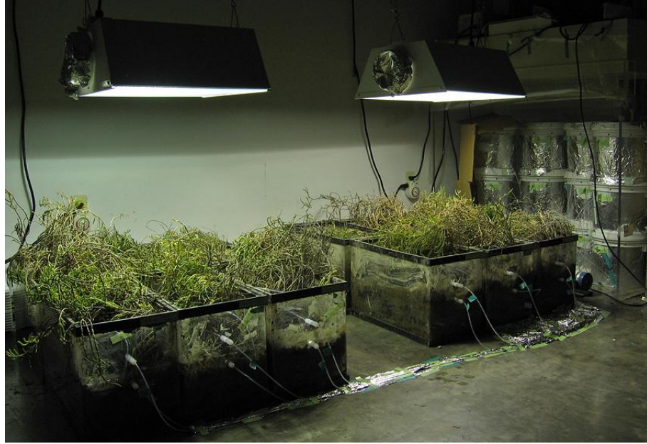
Figure 1. Laboratory microcosm setup including acrylic microcosms, fluoropolymer connections and lines, automated grow-lamps and peristaltic pumps, and individual microcosm reservoirs.
