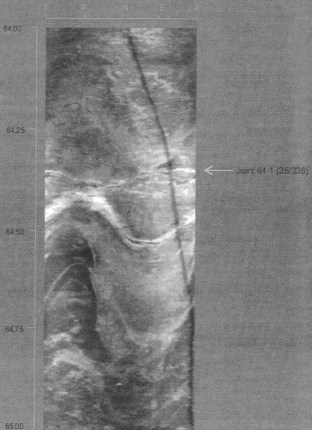
Figure B.13: Unrolled borehole wall image of 64 m. interval
