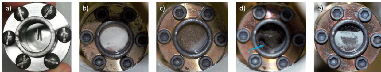
Figure 12 – Test of the sapphire window with LiCl-KCl (40 hrs at 400 °C) and a AISI 304 sample (Maudlin Products). a) shows the empty chamber through the window where the TC is visible; b) is the chamber filled with salt powder; c) and d) show the salt partially and fully molten; respectively. The blue arrow points to an area where the backside of the sample is visible through the salt, while the rest is covered with opaque corrosion products; e) shows the chamber after the experiment, where the deposit is clearly visible. Note that the salt volume has decreased due to the powder’s low packing fraction.
