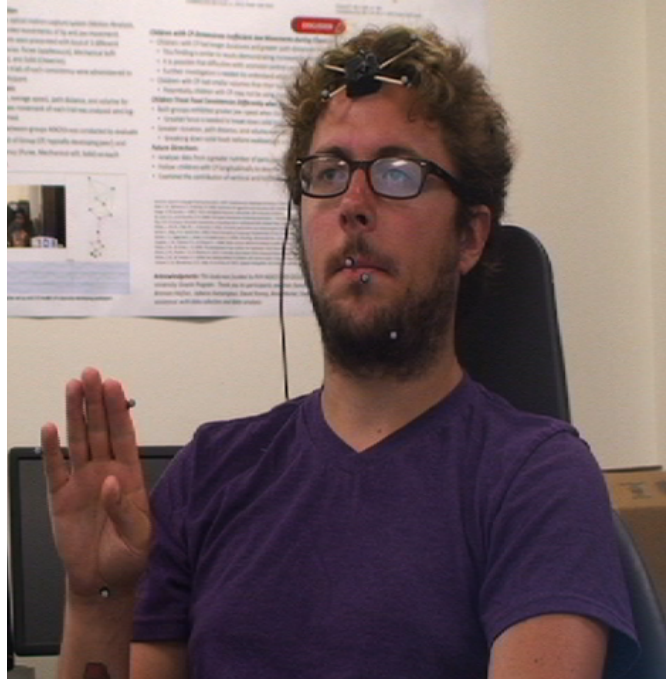
Figure 2.1: Marker placement for data capture. Participants wore a total of ten reflective markers: four on a rigid body attached to the forehead, two on the lips, one on the chin, one on the index finger, one on the pinky finger, and one on the wrist.
