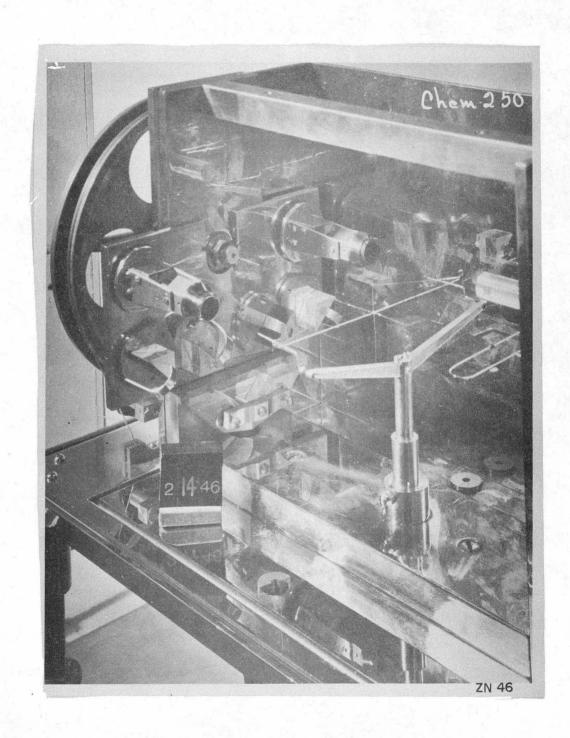
Fig. 5. Quartz fiber torsion balance - interior view.
