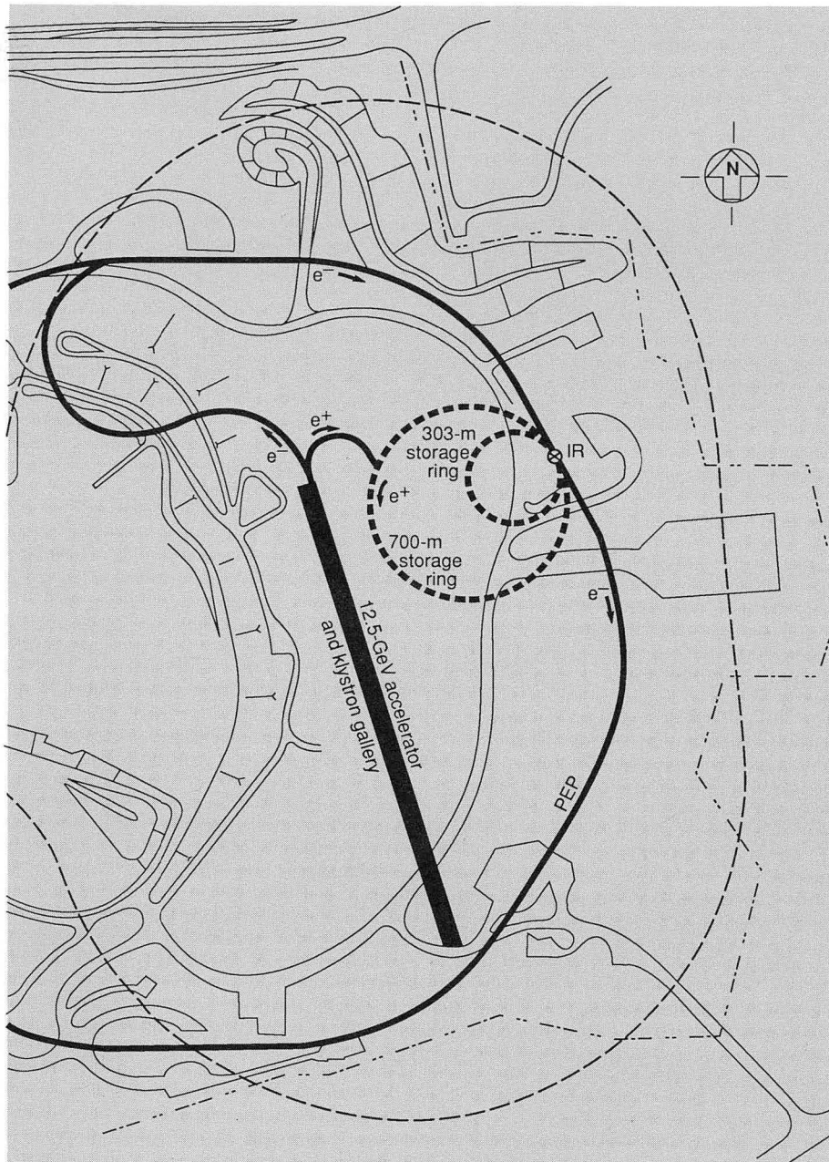
Figure 5-4. APIARY could be built at SLAC with the addition of a 3-GeV storage ring (in either of two physical sizes) near the existing PEP storage ring. Because of the energy asymmetry, the center of mass of the collision moves in the laboratory frame of reference; thus the decay products are separated in space and time, making detection easier.
