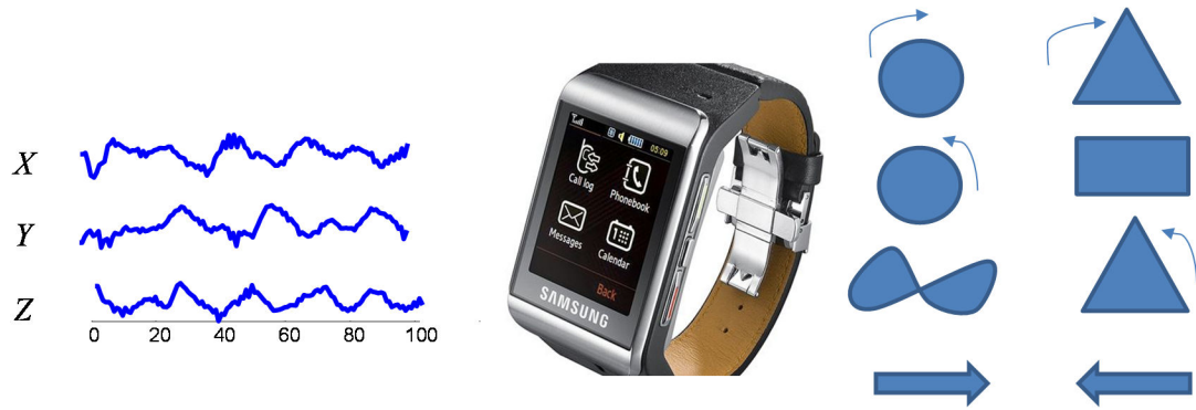
Figure 40: left ) Sample accelerometer data ( X , Y and Z ) of a gesture. middle ) A Samsung Gear 2 used to collect activity data. right ) the eight different gestures considered in our experiments.
