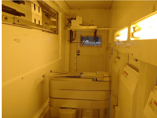
Figure 2.1: A photo of the factory interface with a wafer handling robot.
