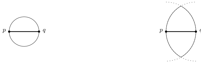
Figure 6.4: The edge between any two points p and q exists, if their “region” is empty, i.e., free of other points. Left: For a Gabriel graph, the “region” is a circle with an edge (p, q) as a diameter. Right: For a relative neighborhood graph, the “region” is an intersection of two half-circles, with centers at p and q , and a radius (p, q) .
