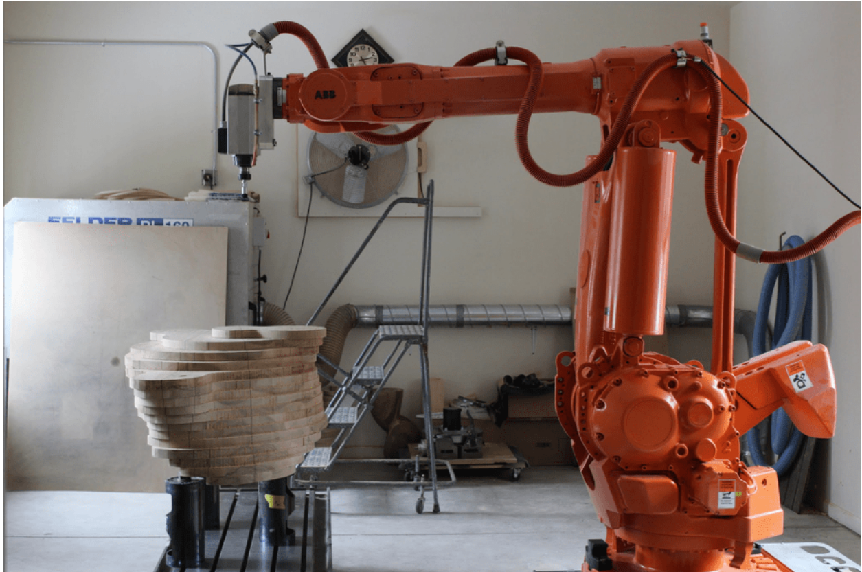
Figure 20 CNC machine fit with a router as it prepares Long Night for milling. Courtesy of Amy Cheatle. Photography by Amy Cheatle.
