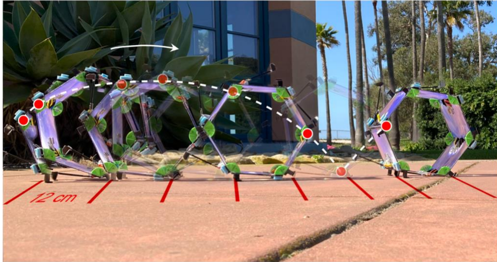
Fig. 9. Demonstration of solar-powered locomotion. The robot was placed outdoors in Santa Barbara, CA and allowed to roll autonomously as it harvests sunlight. This composite figure illustrates the robot completing seven flips, rolling an average speed of 0.764 \text{ cm s}^{-1} using roughly 870 \text{ W m}^{-2} of sunlight (see Supplementary Video 1).
