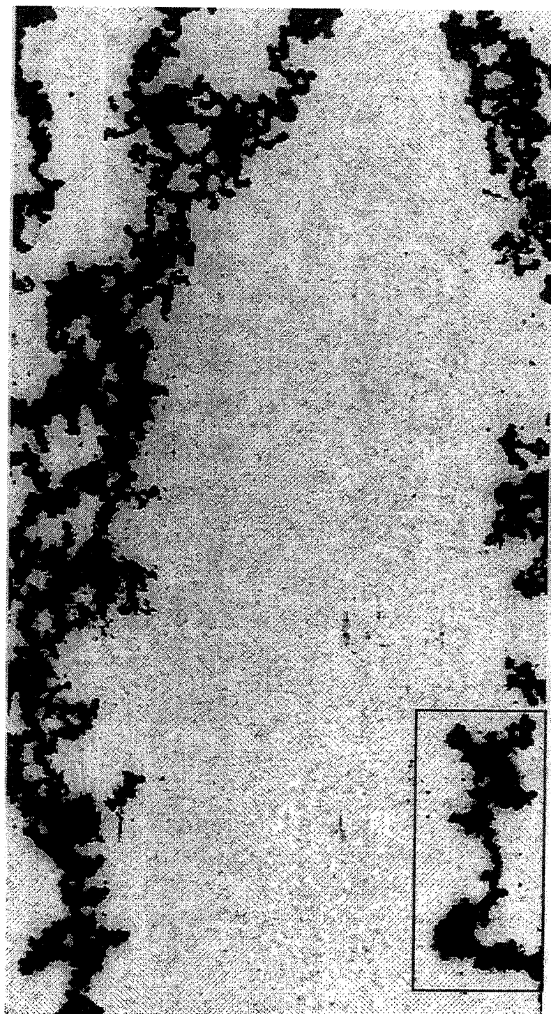
Figure II.B.3: Composite image of buoyant air invasion into a vertical analog fracture: As seen in Figure C-1 air invaded the fracture as discrete bouyant bubbles. As a result, individual images provide little information on air pathways through the system. This composite image was created by summing the changes in phase occupancy for all images collected during this experiment. The paths taken by the bouyant air bubbles are depicted in black, and the zones that remained water saturated as speckled gray. The red box outlines the region enlarged for Figure C-1.
