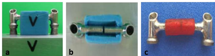
Fig. 2 a, b Silicon model to standardize resin volume. c IFPD indexed with acrylic resin
