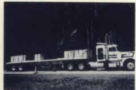
Fig. 4 Experimental Vehicle, a Peterbilt 359 truck
