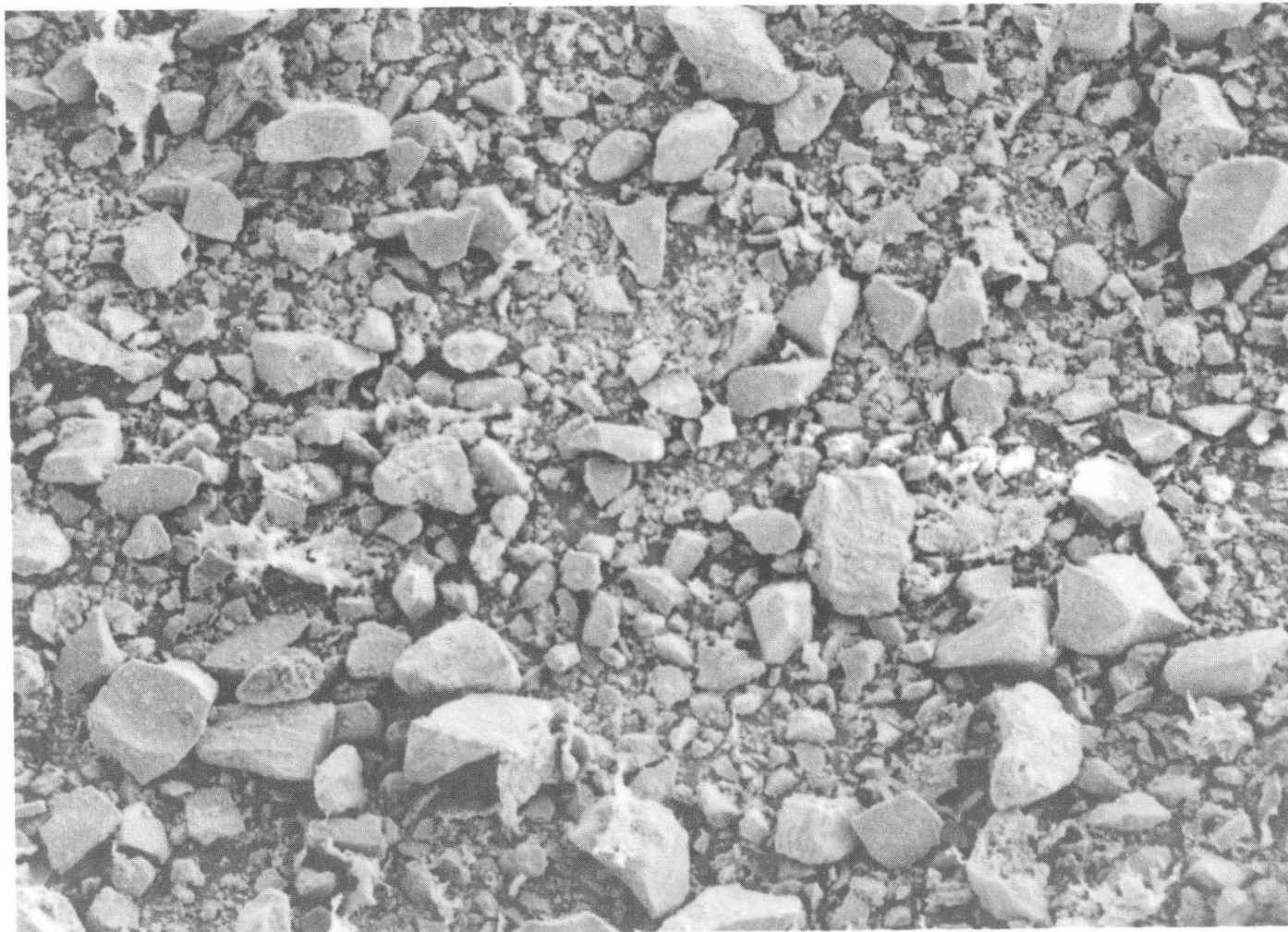
Figure 6 SEM Micrograph of Unfired Mixed Powder
