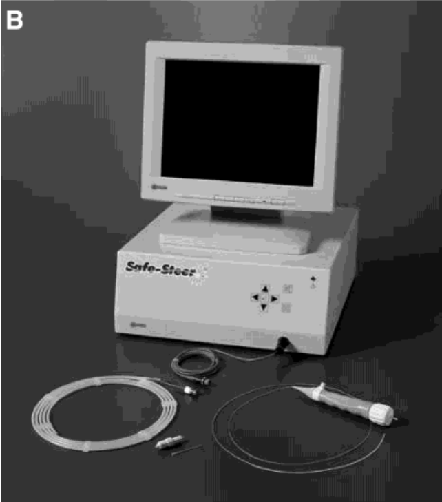
Fig. 1. A: Schematic diagram of the optical coherent reflectometry (OCR) system. The area enclosed with the dotted line represents the components within a console unit. There is only a single fiber that extends from the console that is integrated in the OCR guidewire. B: The console and guidewire control system.
