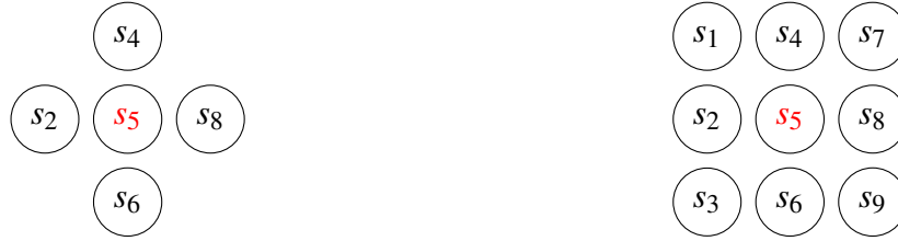
Figure 5.2. Local pixel neighborhood in 2D. The partially and fully connected neighborhoods are shown on the left and right respectively. The point s_5 (colored in red) is considered a local maximum if its value is larger than its neighbors.
