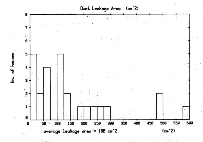
Figure 2: Duct Leakage Area Measurements (cm<sup>2</sup>) for houses tested in component leakage and Atlanta studies
