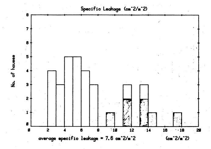
Figure 1: Specific Leakage Areas (cm<sup>2</sup>/m<sup>2</sup>) for houses tested in component leakage and Atlanta studies. Shaded portions represent Atlanta houses.
