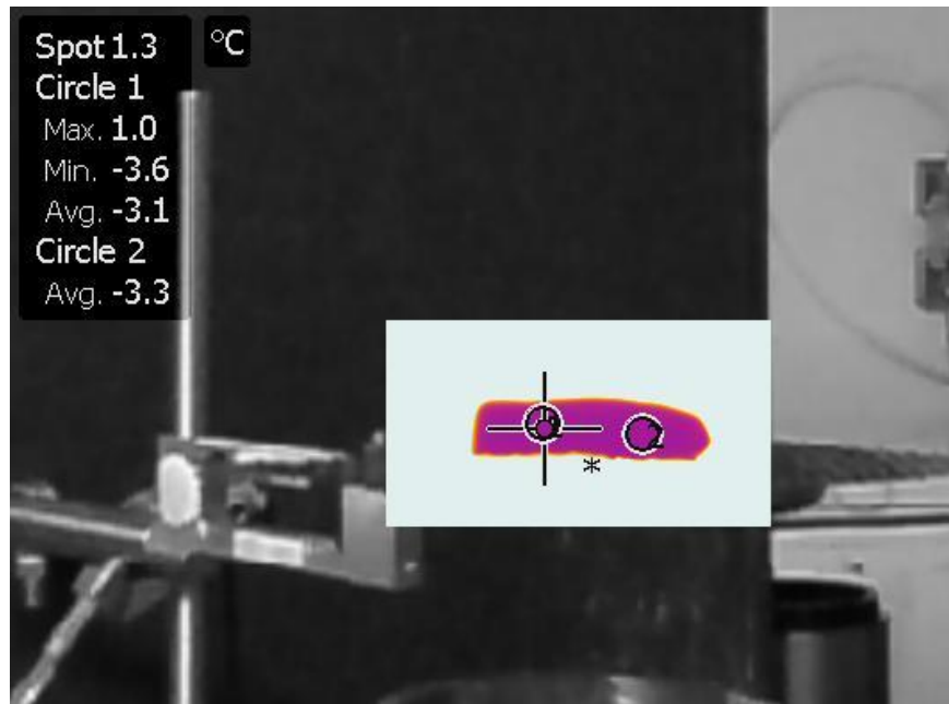
Figure 29. Measurement of methane hydrate temperature after 20 minutes.
