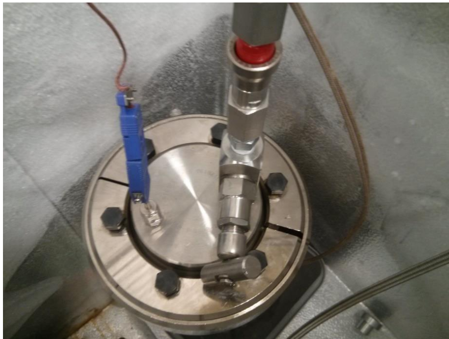
Figure 21. Pressure cell inside the freezer.
