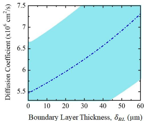
**Figure 2.** The diffusion coefficient calculated from Eqn. 12 for the conditions  $\mathbb{P} = (2.7 \pm 0.1) \times 10^{-4}$  cm/s,  $\delta_m = (63.9 \pm 0.8)$   $\mu\text{m}$ ,  $K_m = (0.31 \pm 0.06)$ . The light blue region represents one standard deviation of the diffusion coefficient, calculated from the propagation of the standard deviations of the individual terms.
