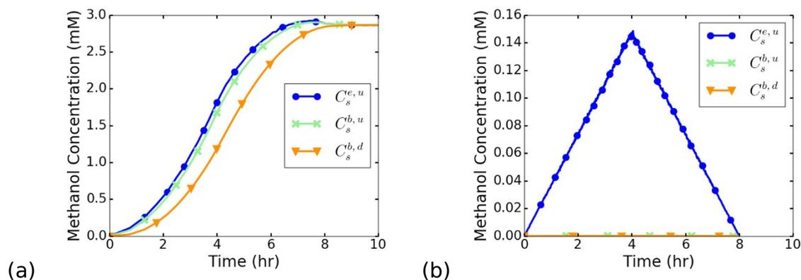
**Figure 7.** Time-dependent methanol concentrations within a solar-driven  $\text{CO}_2$  reduction device (a) without flow and (b) with flow. The blue dots are for the solution within the boundary layer next to the cathode,  $C_s^{e,u}$ . The green x's are for the upstream bulk,  $C_s^{b,u}$ . The orange triangles are for the downstream bulk,  $C_s^{b,d}$ . Note that the vertical axes are not on the same scale.
