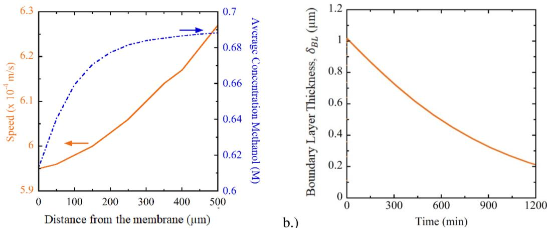
**Figure 4.** (a) The average speed of the solution and average concentration profile in the neck region of the upstream cell at  $t = 600$  min. based on distance from the membrane. (b) The mass transfer boundary layer thickness,  $\delta_{BL}$ , calculated from Eqn. 18 as a function of time.
