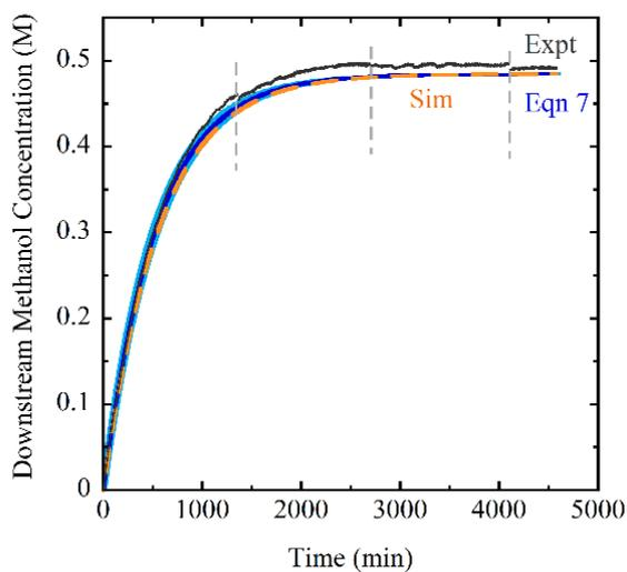
**Figure 3.** Time-resolved downstream cell methanol concentration for permeation through Nafion 1100: experimental results (black), the fit of Eqn. 7 to experimental data (blue), and simulation results (orange). Vertical dashed gray lines are the times at which a fresh background for the FTIR probe was collected. Error (light blue) associated with the fit of Eqn. 7 represents 1 standard deviation from the average  $P_m$ , which is barely larger than the linewidth.
