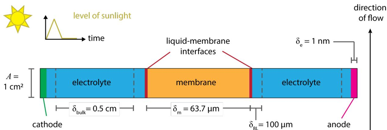
**Figure 6.** Diagram (not to scale) of a solar-driven CO<sub>2</sub> reduction device and setup for the multiscale model.
