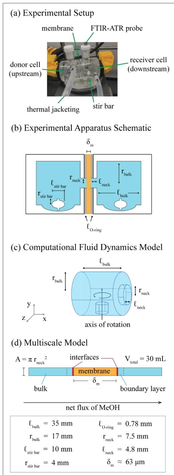
**Figure 1.** The (a) experimental setup (showing one FTIR probe, experiments were also conducted with FTIR probes in both upstream and downstream cells) and (b) experimental apparatus schematic are used to determine the geometry of the (c) cell in the CFD simulation and the (d) multiscale model. Relevant dimensions are shown at the bottom of the Figure.
