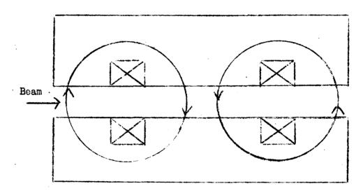
This magnet would weigh about 25 tons and would probably be driven externally with simple harmonic motion as it moved in and out on tracks.
