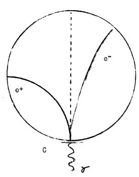
resolution around the circumference can be calculated or corrected by varying the geometry of the detectors. A 1.5 Bev electron is deflected 26° in a field of 20 kilogauss, in the 40-inch magnet.
