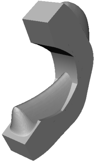
Figure 8. Sweeping the generator of Figure 6 along a semi-circular arc. The generator is tumbled as it is swept.
