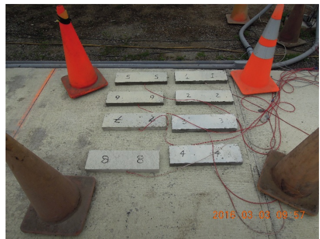
Prisms after demolding
