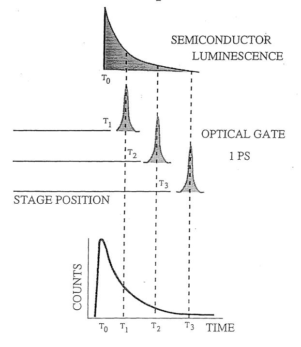
Introducing a variable path length is trivial, for example, 1 ps corresponds to a .3 mm distance. Controlling even micron distances with commercially available translation stages is routine. Hence, achieving the picosecond resolution is not difficult. The difficulty lies in generating the upconverted signal itself.
