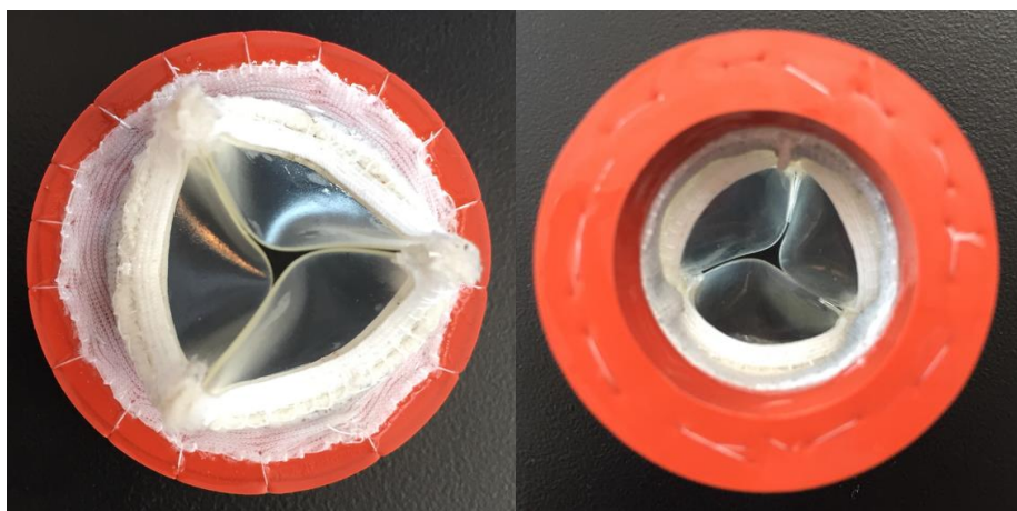
Figure 4.6 After 10 million cycles, the valve showed an uneven, spiral-like coaptation. This is likely due to asymmetrical sewing of the leaflets to the posts and frame.
