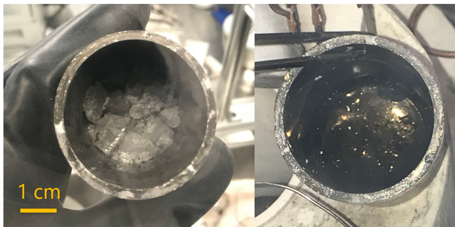
Figure 1.1. FLiBe + 0.8 mol% LiH at room temperature (left) and at 700°C (right).
