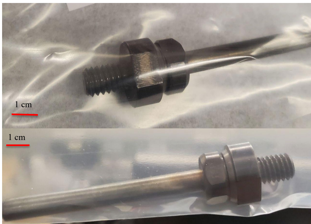
Figure 2.3. FLiBe in vanadium PAC can with graphite gasket and Ti lid prior to heat testing under vacuum in preparation of the NOMAD 2022 experiment. Photos by ORNL staff researchers.
