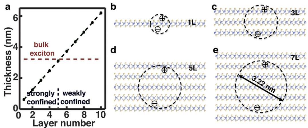
**Figure 4. Geometric confinement of excitons in MoS<sub>2</sub> films.** (a) Comparison of the size of the exciton in bulk MoS<sub>2</sub> with the thickness of MoS<sub>2</sub> films. The regime where the film is thinner than the exciton size is categorized as strong confinement. (b–e) Schematic illustration of the size of excitons in the films with different layer numbers.
