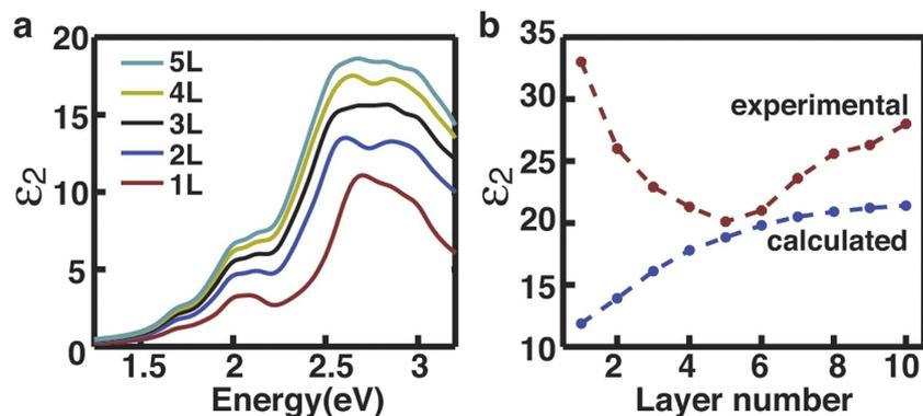
**Figure 2.** Comparison of the measured and calculated dielectric function of 2D MoS<sub>2</sub>. (a) Calculated imaginary part  $\epsilon_2$  of the dielectric function of MoS<sub>2</sub> with different thickness. (b) Comparison of experimental and calculated results for  $\epsilon_2$  at the C peak as a function of the layer number. The error bar in the experimental result is ignored for visual convenience.
