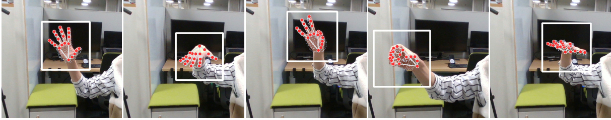
Figure 2.4. Hand Pose Detection Visualization. This figure visualizes the hand detection results, with the white bounding box highlighting the predicted area and red points marking the identified finger key points. The hand skeleton is represented by the grey lines connecting the key points. Additionally, the small grey points depict the 2D projection of 3D vertices from the SMPL-X hand model. The figure showcases five diverse cases, from left to right: (i) a hand spreading out the fingers to initiate teleoperation, (ii) fingers facing downwards in preparation for a top-down grasp, (iii) a precision grasp using the thumb and index finger, (iv) a power grasp using all five fingers, and (v) a failure scenario where the hand is positioned vertically relative to the camera plane.
