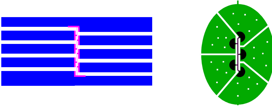
Figure 3.12: Left: Example of an old CDMSII era QET that can be described by a 1D diffusion model. Figure from [76]. (Blue is Al, pink is W). Right: A more modern elliptical QET design from SPICE that is better modeled with a 2D diffusion model. (Green is Al, purple/black is W)
