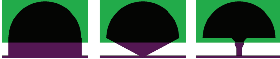
Figure 3.16: Schematic showing conceptual fin connector designs (the purple region connecting the black overlap region to the purple TES). Left: most efficient from QP transport perspective, but poor noise performance. Middle: Idea to ‘funnel’ QPs to TES, while reducing the W volume of the design on the left. Right: Actual fin connector design from a SPICE QET, where the bulk of the fin connector has been made as narrow as possible, but the funneling concept of the middle idea has been incorporated into the W/Al area part of the connector.
