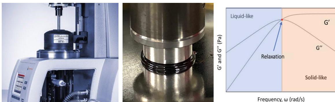
Figure 1-6 From left to right: picture of the Anton Paar MCR 92 rheometer with parallel-plate and Peltier heater setup, sample geometry in a shearing experiment with parallel-plate setup, typical G' and G'' spectrum as a function of oscillatory frequency.
