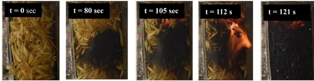
(B): Smoldering to flaming transition ignition in shredded avena fuels.
